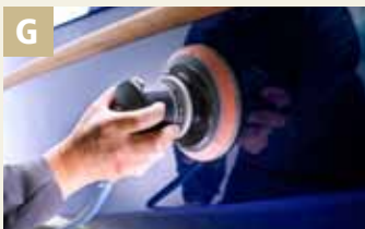
G Microfinishing prior to polishing
