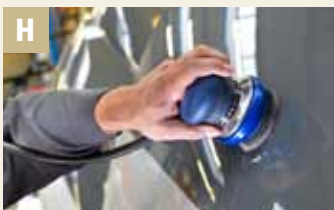
H Microfinishing prior to polishing
