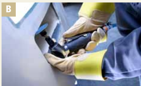
B Deburring of edges in hard-to-reach places
