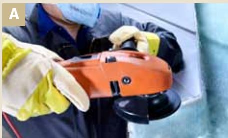
A Deburring the casting mould edge
