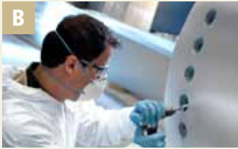
B Deburring of drilled holes, adjusting drilled holes to size
