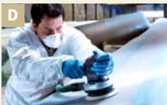
D Sanding out defects such as «pinholes»
