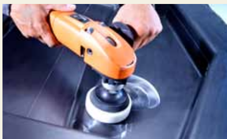
Polishing the basic mould
