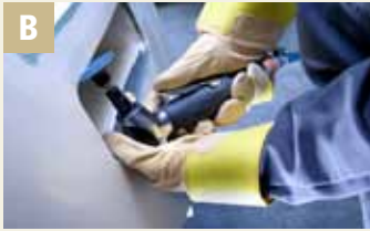
B Deburring of edges in hard-to-reach places
