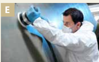
E Keying/flat grinding of rough surfaces
