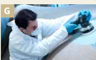
G Flat grinding/ fine sanding of epoxy filler
