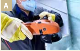
A Deburring the casting mould edge
